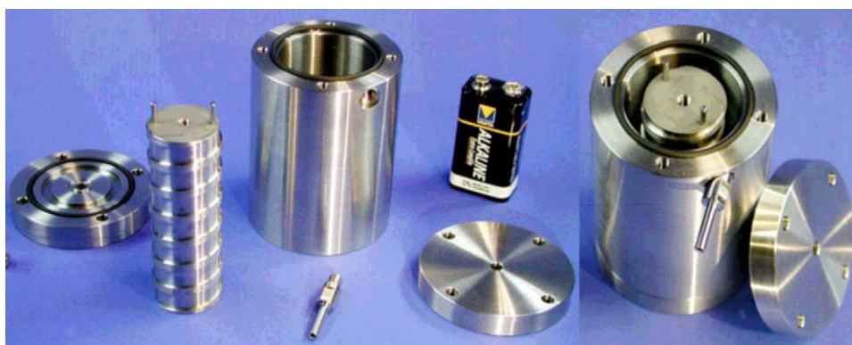
Fig. 6. New helical falling film micro-reactor with an extended path length of 540 mm.
